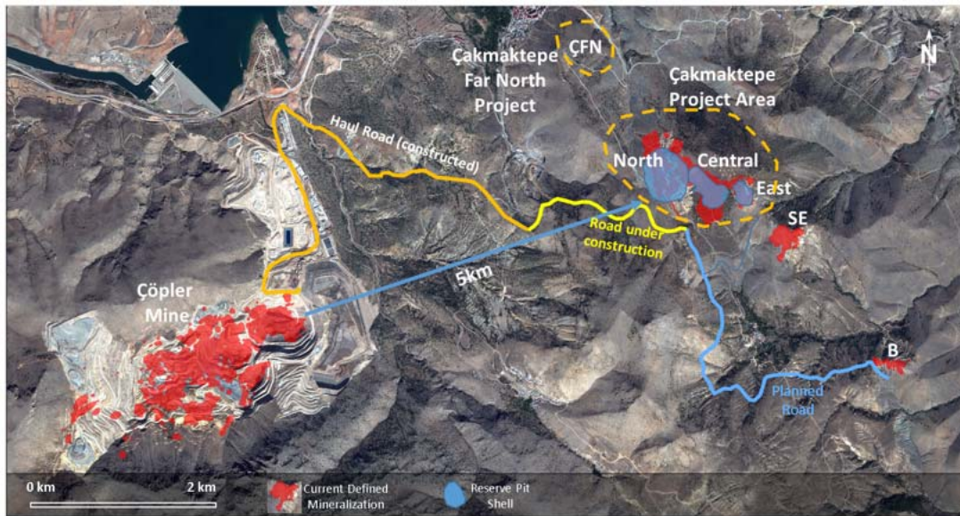
Çakmaktepe Prospect Location Plan: Çakmaktepe Project: North, Central, East and Southeast; SE = Çakmaktepe Southeast; B = Bayramdere. Red outlines define mineralization envelopes. Blue shapes define resource pit shells. ÇFN: Çakmaktepe Far North exploration property.
